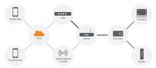
Gallagher SMB uses cloud architecture, requiring no server to be installed on-site. The system is designed to be plug and play - once powered on, the controller will automatically assign an IP address using DHCP, download a default configuration and update itself with the latest firmware, cyber security, and functionality.
